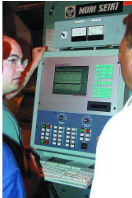
A two-axis Mori Seiki lathe makes a retrofit every bit as neat and easy as the more-common machining center retrofits. Control software typically covers both
