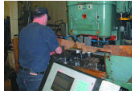
The old control on this twin-spindle Matsuura VMC was hard to keep running, too slow, and had insufficient parts-program storage. A modern PC solved all three problems
