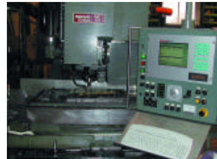
A 3rd party add-on program gave this Knoxville-area jobber conversational programming for programming at the control. Flexibility to handle add-ons is a big advantage of PCs' open architecture
