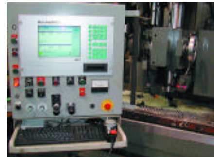
Monarch VMC retrofitted with a MachineMate MM1, a low-end Windows NT-based control, performs all of the functions of the CNC it replaces, and more
